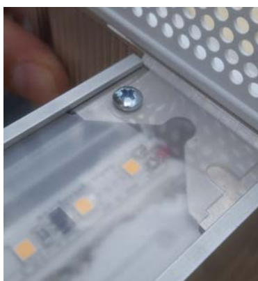
7B. To remove lens: Insert flat blade along side near end to cause lens to bow; then pull lens free.
