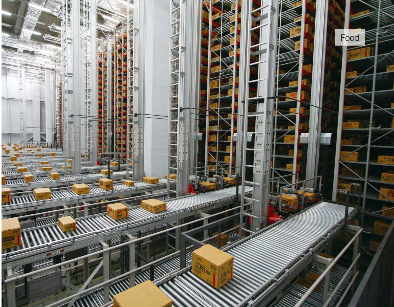
Mini Load system with 18 cranes and over 50,000 storage positions—supporting high-volume confectionery distribution operations
