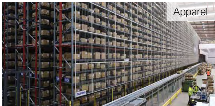
130-meter-long, double-deep AS/RS with over 76,000 storage locations—designed for a leading workwear apparel company
