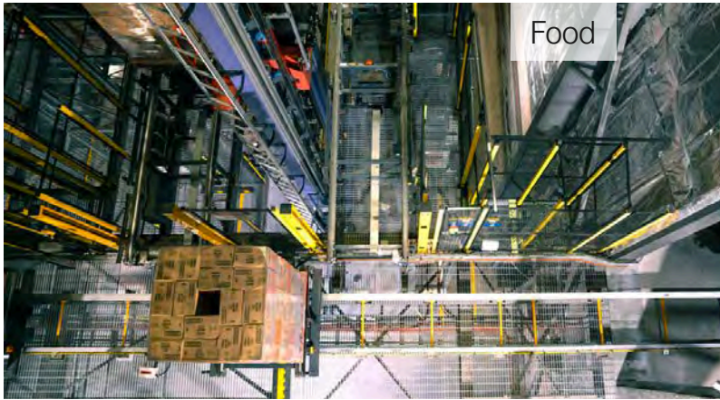
Food An STV loop transports pallets between multiple processes—storage, case picking, and shipping.
