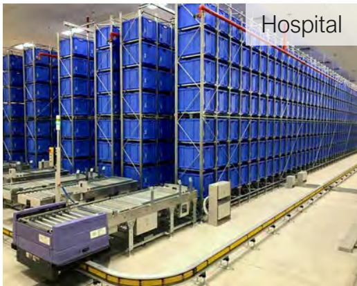
A Mini Load AS/RS combined with mini STVs ensures timely tote delivery to goods-to-person stations.
