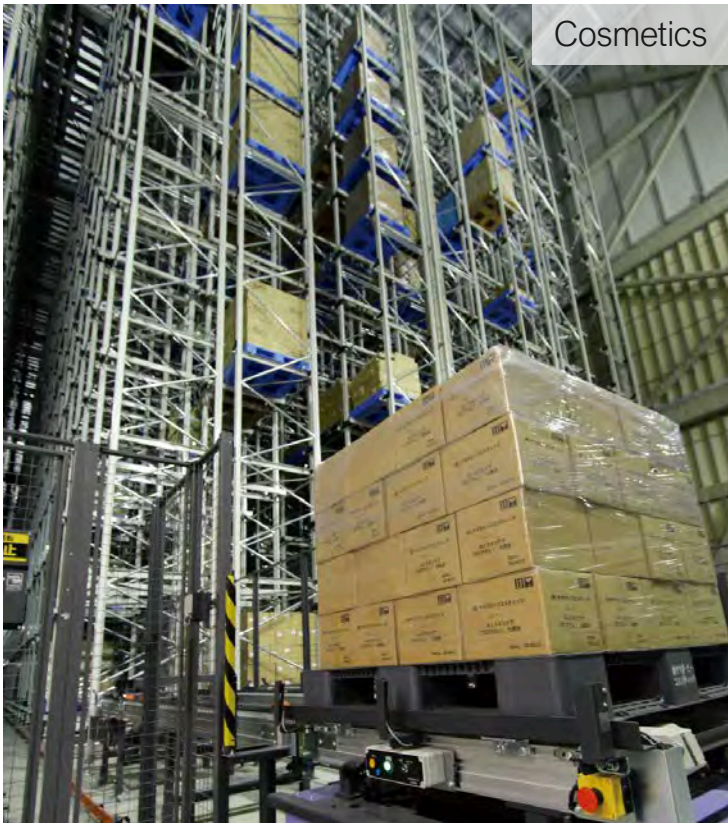
Cosmetics Transporting palletized finished products to a Unit Load AS/RS until called for shipping.
