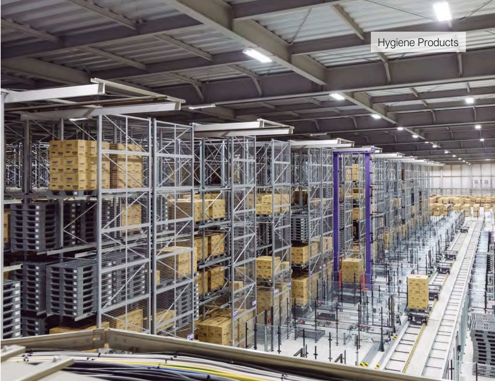
Hygiene products stored and staged for shipment, with final sorting handled by an STV loop
