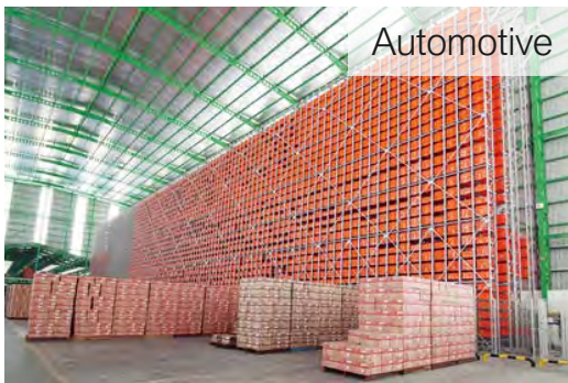
15-meter-high AS/RS system capable of storing over 14,000 containers of motorbike parts
