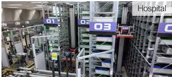
Mini Load storing sterilization containers with surgical kits in a hospital
