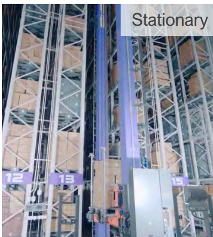
Unit Load stacker cranes handle pallets of stationery products, supporting high-volume distribution
