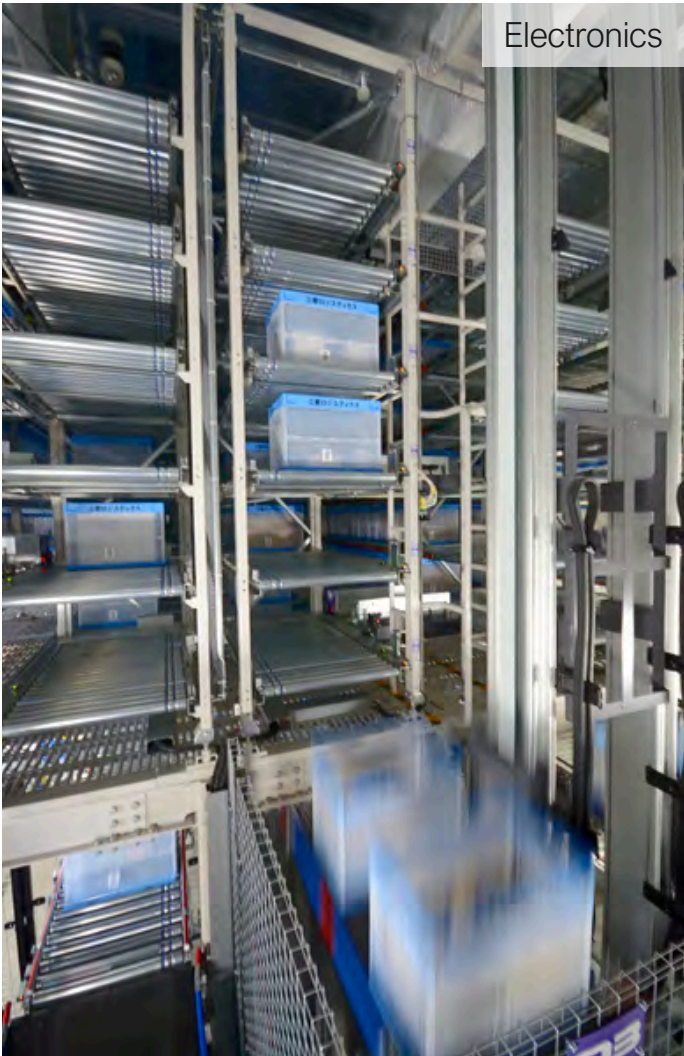
Lifters facilitate the movement of electrical appliances between levels for a major camera manufacturer
