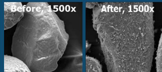
Nanocatalyst deposition observed to be localized on surface of sand face where the dispersed nanoparticles are observed to be much smaller than pore throats.
