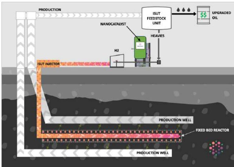
**Two stage process: one-time preparation phase establishes the nanocatalyst bed, and a cyclical upgrading and recovery phase.**
