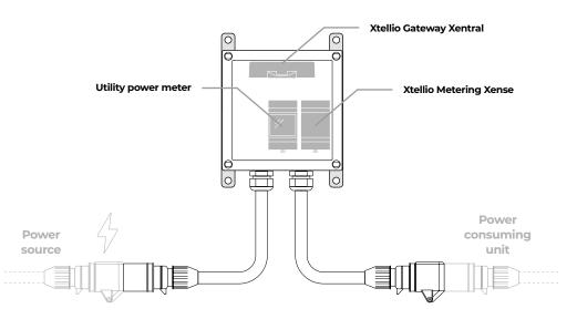
Plugged in between the power source and your power-consuming unit, the Xtellio Remote Power Kit reads precise power consumption data (kWh) from a built-in utility power meter.
