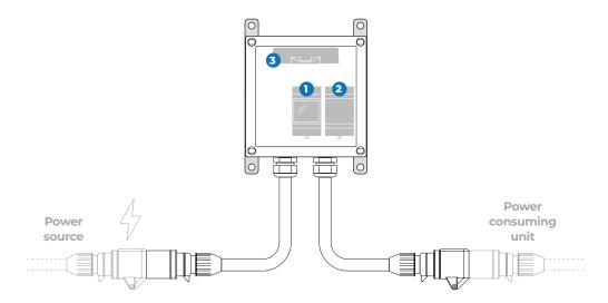
Plugged in between the power source and your power-consuming unit, the Xtellio Remote Power Kit reads power consumption data (kWh) from a built-in utility power meter.
