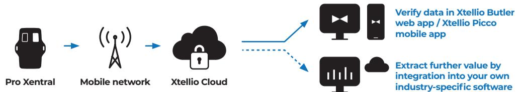
All collected data is transmitted securely to the Xtellio Cloud via a built-in SIM module, which utilizes NB-IoT or LTE-M networks (with 2G fallback) for robust performance, even in areas with limited coverage.
