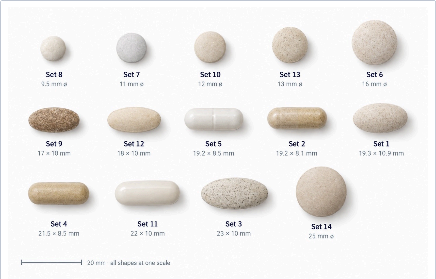
Figure 2 — the pressed tablet from each tooling set, one common scale, smallest to largest. Shown face-on as it leaves the press, uncoated; the set numbers in the artwork are our tooling references. The 25 mm round is drawn under the common scale — read its diameter from the table, not from the picture.
