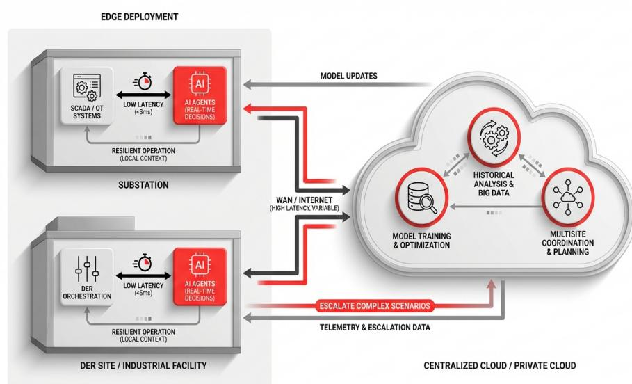
Hybrid edge-cloud architecture enables millisecond-latency decisions at operational sites while leveraging centralized compute for complex analytics and model training.
