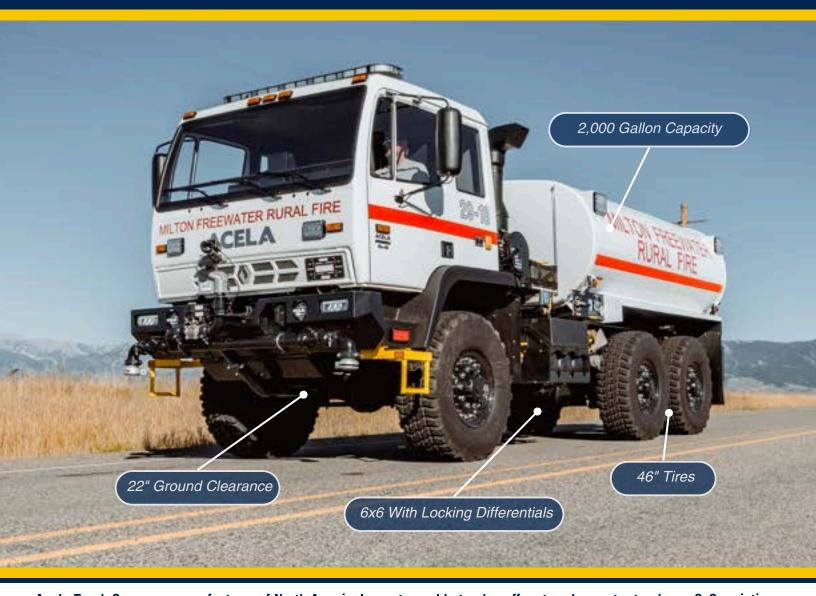
Acela Truck Company, manufacturer of North America's most capable trucks, offers turn-key water trucks on 6x6 variations of its Monterra™ line of truck chassis. With 47-inch tires and 22-inches of ground clearance there is no other modern truck platform that can compete when it comes to reliable and safe operations in construction and civil projects.
