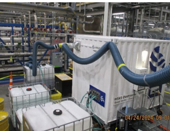
Commercial-scale HALT system operating at a water quality building during a 2-week pilot trial.
