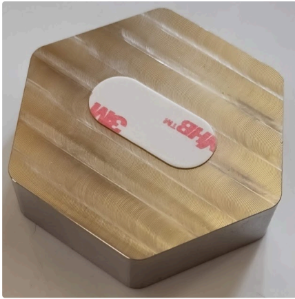
a. Mount with small VHB installed
