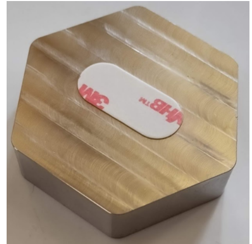
Step 2: the surfaces are prepped and the VHB has been applied to the center of the case, covering up the screw mounting holes.
