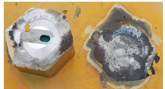
Step 2 Figure 2: Example of a poorly prepared surface that resulted in pre-mature failure. The surface was not properly ground leaving residual rust and paint causing poor adhesion. You do not want your surfaces to look like this, instead you want them to look like above in Step 2 Figure 1.
