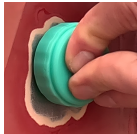
Step 4. Press firmly on the product for 15-to-30 seconds to activate the VHB adhesive.
