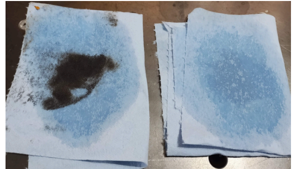
Step 3: Continue cleaning until the rag is still clean after wiping like shown on the RIGHT above (i.e. the rag is wet with Isopropyl Alcohol but no dirt or grease). If after wiping the rag is dirty like shown on the LEFT above, you need to continue cleaning and wiping.
