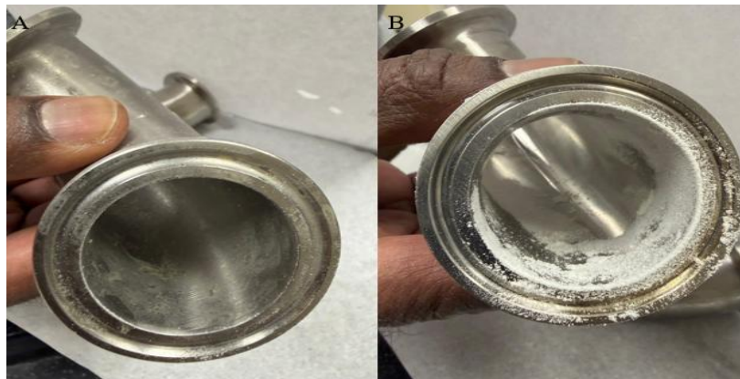
Figure 4. Residual after compressed air application of the coated elbow and the uncoated elbow. A = Interior surface of the elbow coated with whey protein–starch matrix, and B = Uncoated elbow used as control.
