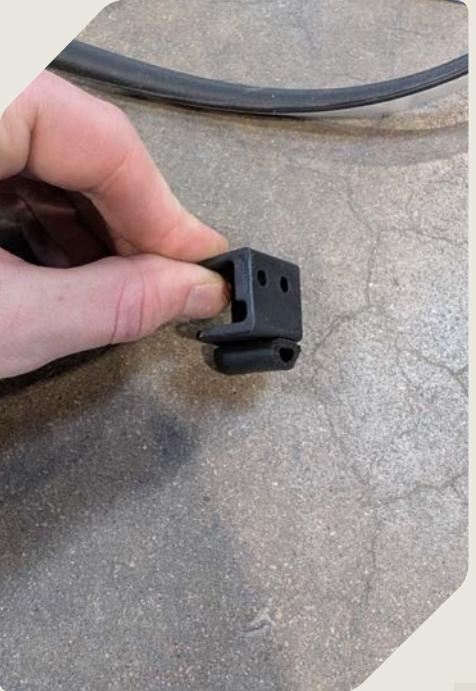
1. Attach the d-bulb to the underside of the rear door gap filler
