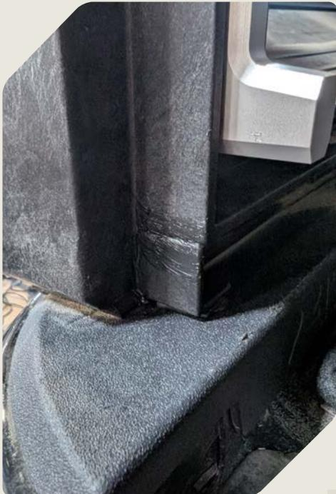
1. Clean up excess silicone squeeze out with a rubber glove or rag
