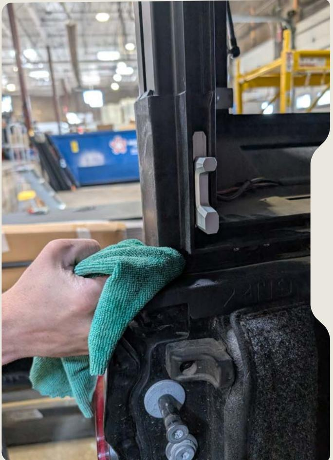
1. Once the drill template is removed clean the area again with isopropyl alcohol, taking care to remove all debris from the area
