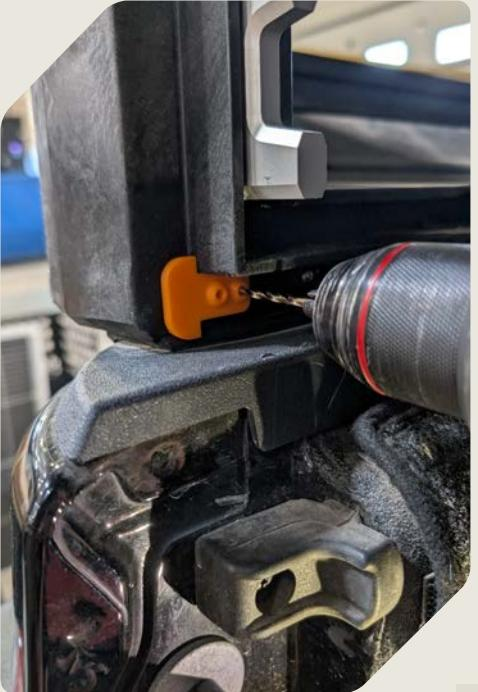
1. Drill a hole in both locations on the drill jig using a  $\frac{1}{8}$ " drill bit
