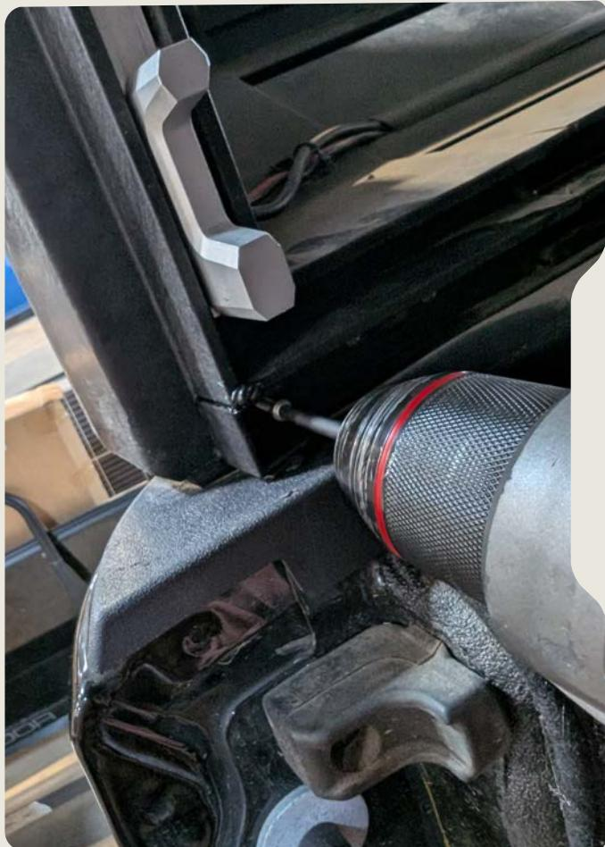
1. Secure the rear door gap filler with two plastic tapping screws using the included T20 bit
