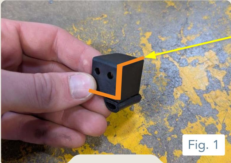
1. Apply a continuous bead of caulk in the area shown in orange (Fig. 1)
