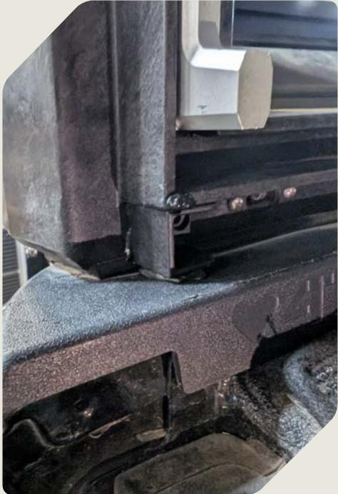
1. Firmly press the rear door gap filler into place while keeping the holes aligned (Fig. 1)
