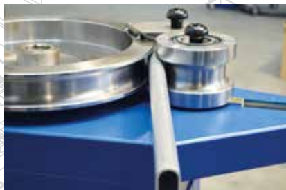
Oval tube bent on device 6000
