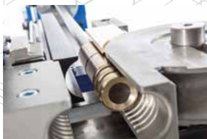
Mandrel bending tool with ball mandrel, crease smoother and travelling slide rail
