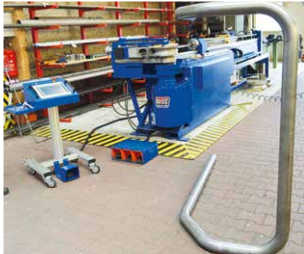
Bending capacity up to 100 mm possible with the mandrel bending device 9000
