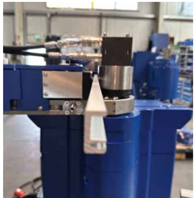
Special construction with automatic opening of profile tools
