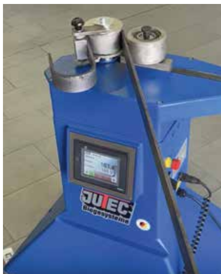
Machine 6000, profile 50x8, centre radius 60 mm
