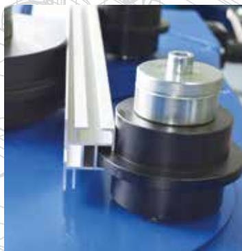
Section tube with special tool on RB60
