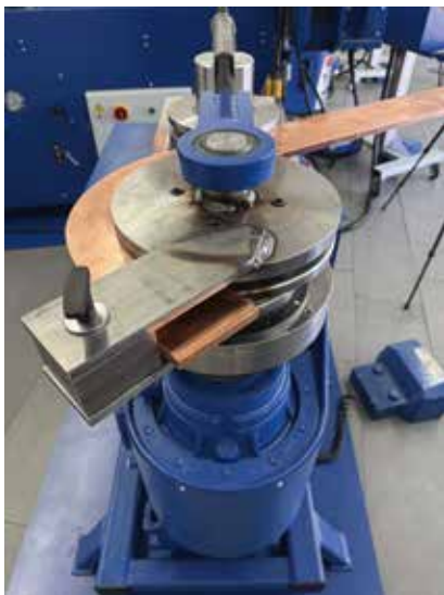
Profile 100x12, inner radius 100 mm
