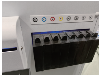
Refillable ink cartridges with ink lack sensor
