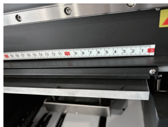
Platform with ruler, easy to set the start origin
