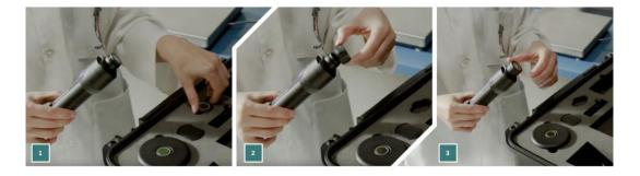
It is important to always screw the adaptor to the same point on the device because a difference in the positioning of the adaptor can lead to variations in the spectra obtained.
