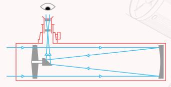
For the reflector telescope light bounces off a concave (primary) mirror, and converges into one point.
