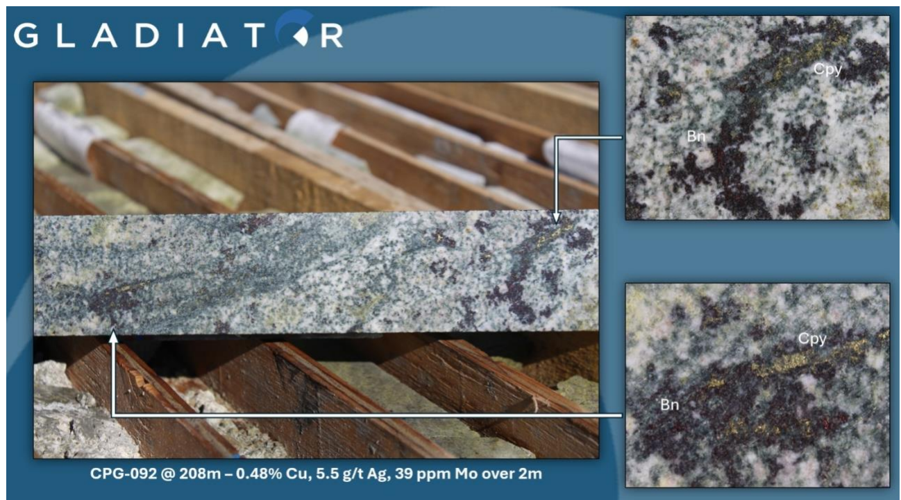
Figure 2: Granodiorite hosted mineralisation in CPG-092 showing disseminated and blebby bornite and chalcopyrite mineralisation replacing chlorite altered mafic mineral component. Patchy epidote alteration also visible.
