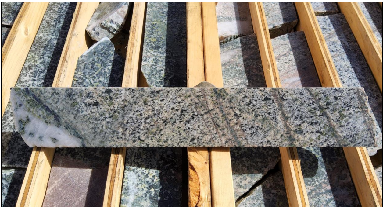
Photo 1: VLG-001D2 164.2-164.5m – Quartz molybdenite veining with potassic alteration selvages within medium-grained, equigranular, epidote altered granodiorite (NTW Core size).
