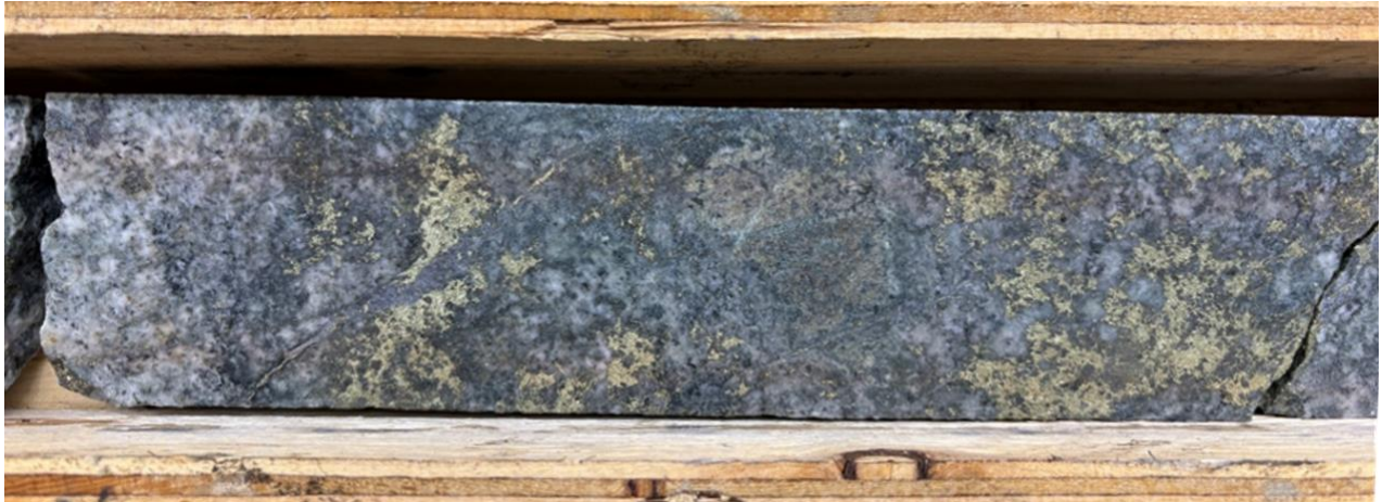
Photo 3: LCG-020 ~306.40 to 306.55m – Close up of brecciated hosted coarse blebby chalcopyrite ± bornite mineralization within brecciated Granodiorite (NTW core size).
