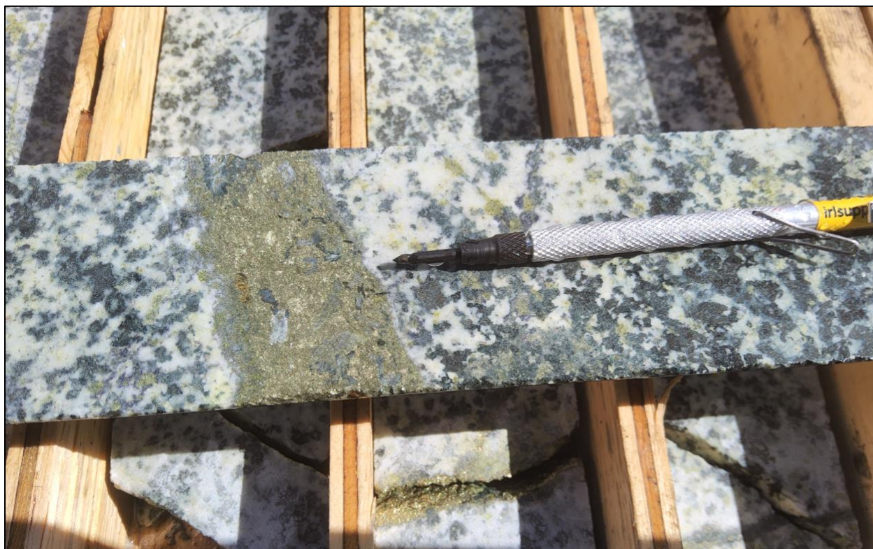
Photo 2: VLG-001D2 216.5-216.7m – Fracture to vein-hosted chalcopyrite mineralization within coarse-grained, epidote altered hornblende quartz diorite (NTW Core size).
