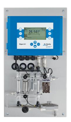
Measuring hydrazine concentrations in high-purity water
