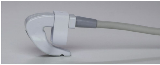
FIGURE 1 | The SIBUS-IN ultrasound probe design. The SIBUS-IN ultrasound probe showing its compact, ergonomic design and fingertip-mounted transducer, optimized for single-handed operation in aesthetic procedures.
