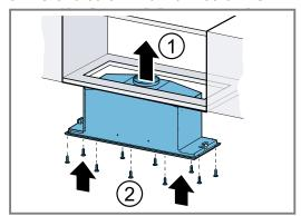
**2.** Tighten the fastening screws.
