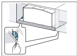
**3.** Attach the frame and screw it to the appliance from
