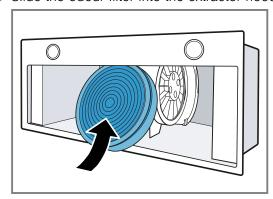
2. Guide the odour filter around the motor.
