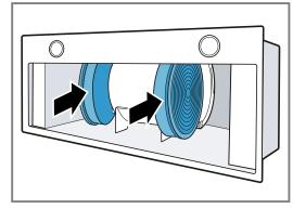
4. Install the grease filters.
