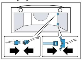
The plug can only be inserted into one position.
