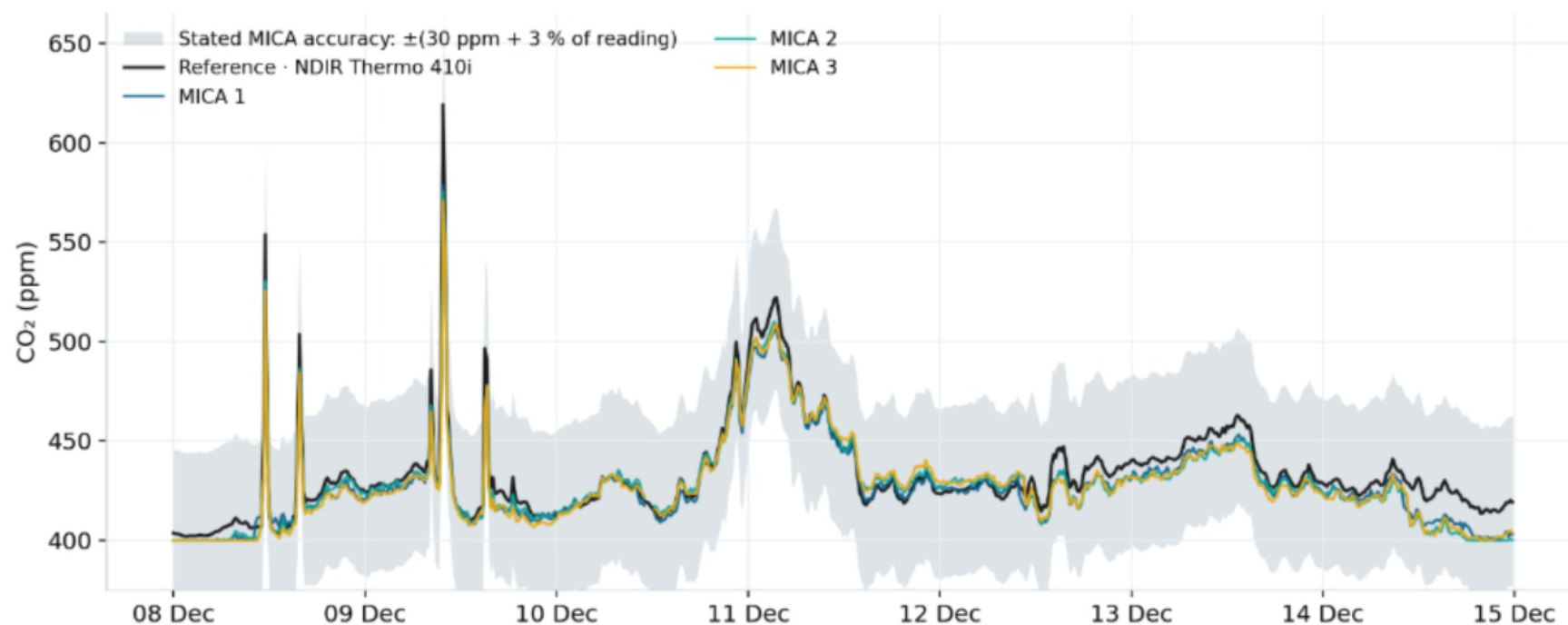
CO 2 against the Thermo 410i reference analyzer · 8 to 14 December 2025
