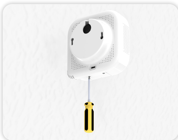
Remove bottom screws (2)
