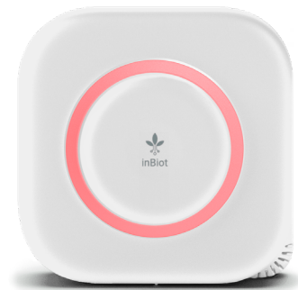
Ventilation is needed
