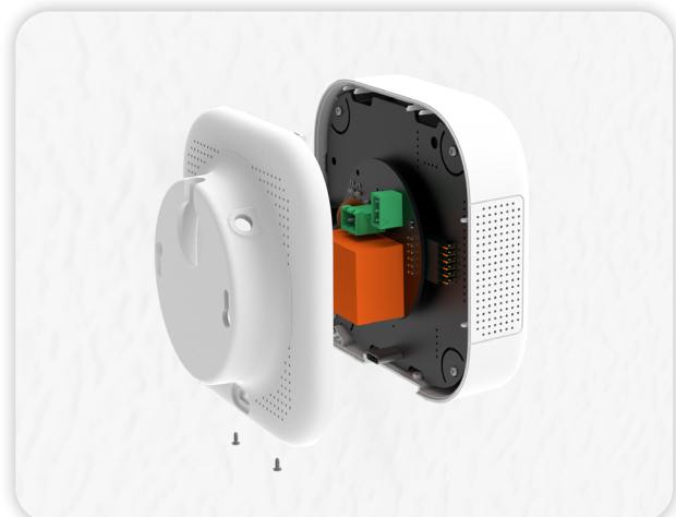
Detach the back cover of the MICA
