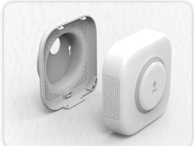
Detach the back cover of the MICA
