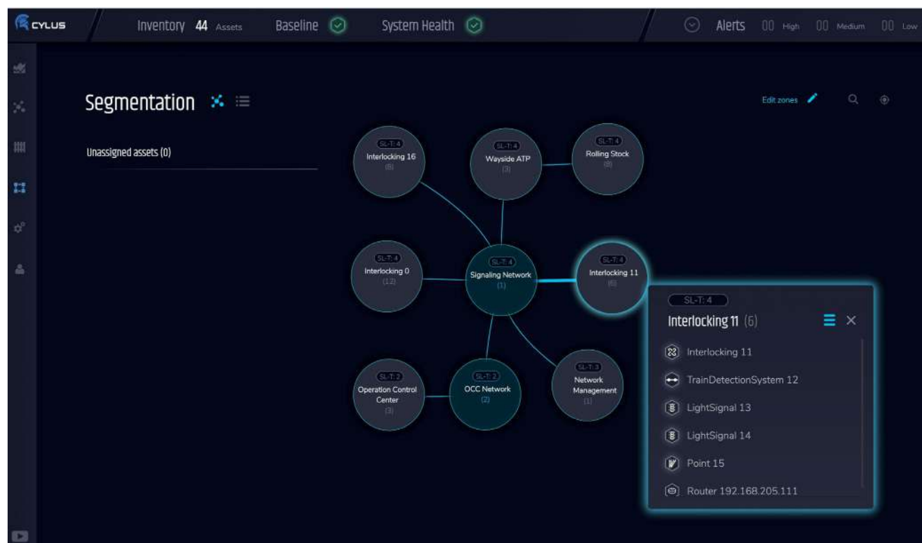
Figure 46: CBTC segmentation per security zones as shown by a Continuous Monitoring System: source Cylus
