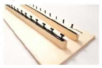
6. After the drying time you can place the sound bars. Clip the oblong holes of the sound bars on the nubs of the clip-on bar and put the sound bars with the round holes between the nubs of the holding bar.
