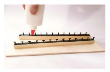
Attach the felt strips on the inside flush on top of the clip-on and holding bars. Cut off the excess of the felt strips using scissors or a knife and let the glue or all-purpose adhesive dry for at least one hour.
