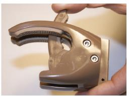
Check 7: Test the movement of one Geared Digit. If it moves smoothly now is the time to REPEAT STEPS 6 & 7 for the other side. Be sure Bolts are tight.
