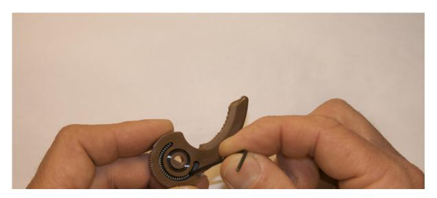
Check 5: Compression Spring is adjusted away from finger end, creating space for the Digit Pin.
