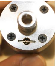
Check 10: Pin should be in Pin Bed and held tightly by the Extension Spring.
