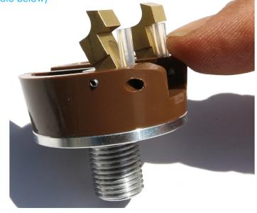
Check 2: Brass Pawls are oriented properly, Roll Pins are pushed in below surface (Sub flush) and Clear Tubes are in position.
