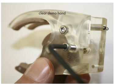
Screw in Side Bolts when two parts are joined properly.
