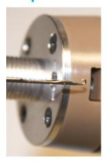
Use the Hook Tool to pull the Extension Spring through the hole in the Plastic and Aluminum Base.
