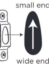
Be sure to place back panel with small end of hook teardrop hole facing up.
