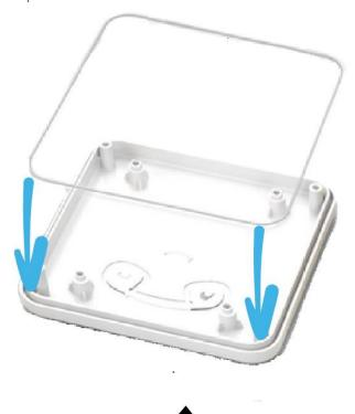
The rubber seal has 4 curved edges that lines up with the lens.
