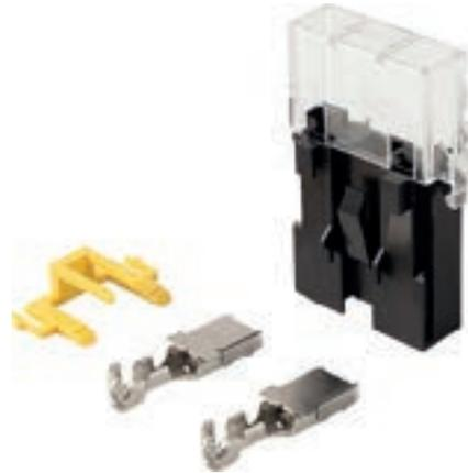
Individual fuse holders. Accepts maxi blade fuses. These splash proof fuse holders can be clipped together to form a multiple fuse block. The fuse holder is supplied complete with cover, terminal locking bar, cable cover and 2 terminals. See **page 49** for FH500P, FH501P and FH502P fixing plates.
