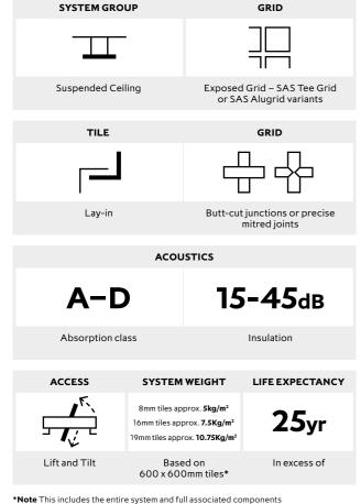
(suspension, tile, acoustic pad and associated fixings.)
