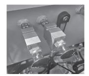
Emergency front and rear stabiliser 'pull' valves.
