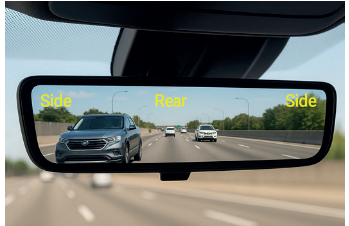
Smart mirror with combined information from different sensors
