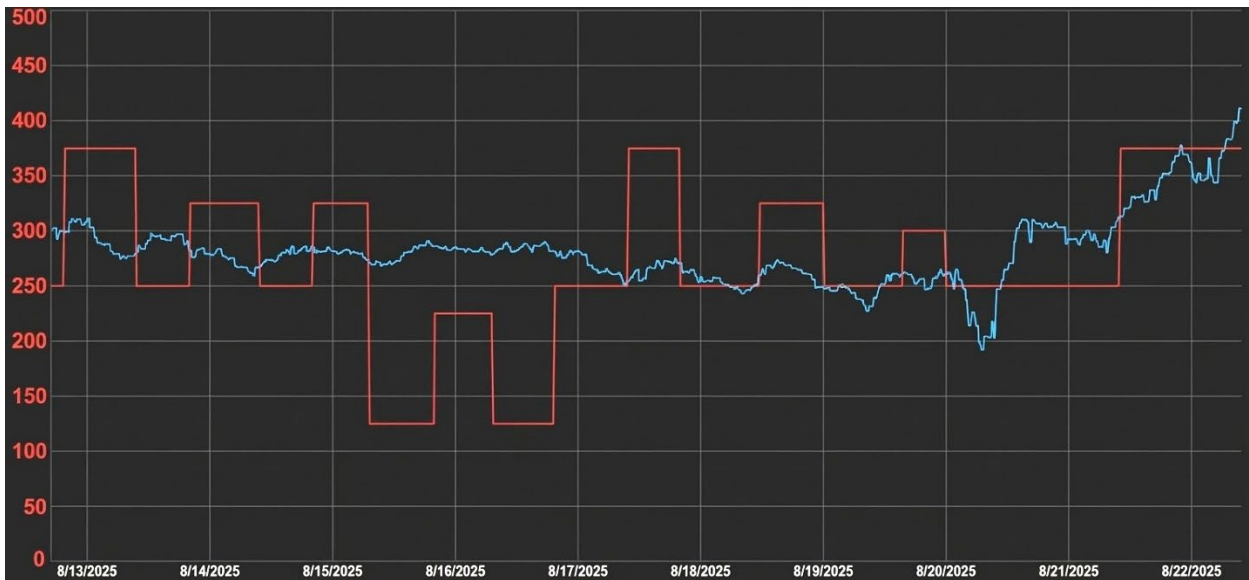
FIGURE 11. CONTINUOUS ANALYZER DATA (BLUE) COMPARED TO LABORATORY GRAB SAMPLE RESULTS (RED OVERLAY), SHOWING PROCESS VARIATIONS INVISIBLE TO PERIODIC SAMPLING.
