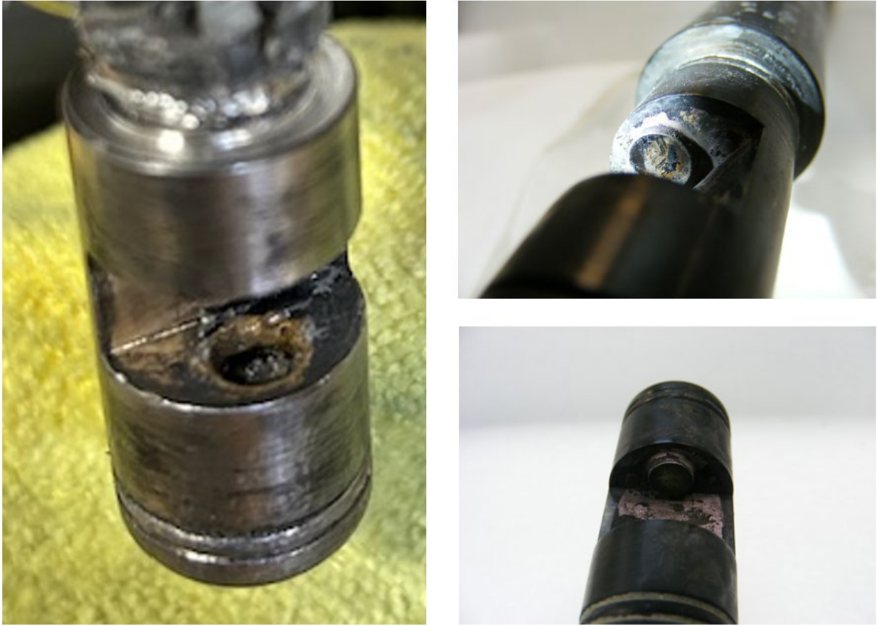
FIGURE 2. FAILED PROBE DUE TO THERMAL EVENT EXCEEDING SPECIFICATIONS
