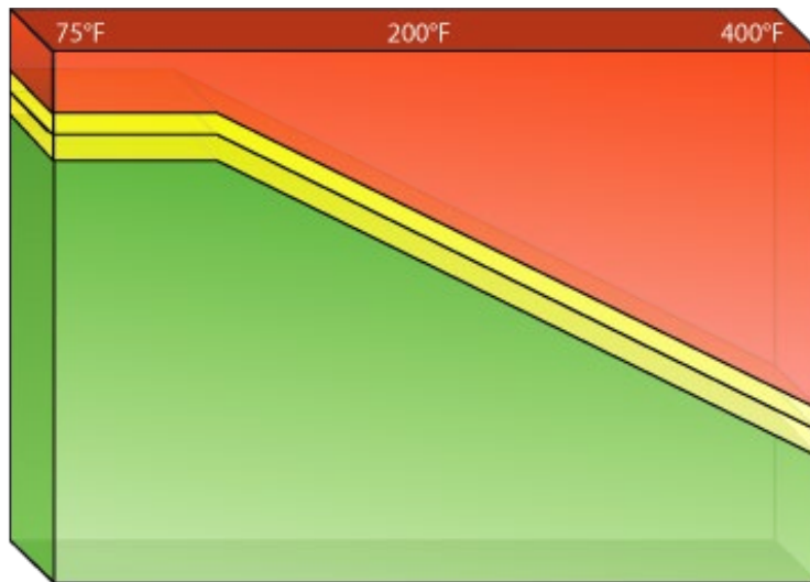
Figure 4. Influence of temperature on flammability limits. Temperature (x-axis) increases from 75–400°F while the y-axis represents vapor concentration relative to the LFL. Increasing process heat can shift a previously safe condition into the flammable region.
