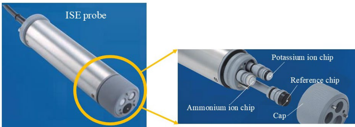
FIGURE 4: PICTURE OF ION SELECTIVE ELECTRODE
