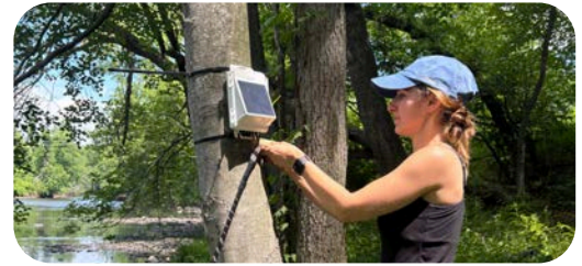
Paige installs a water level station
