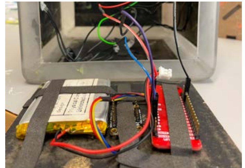
final assembly Mounting the electronics in the cube, including the internal power source.
