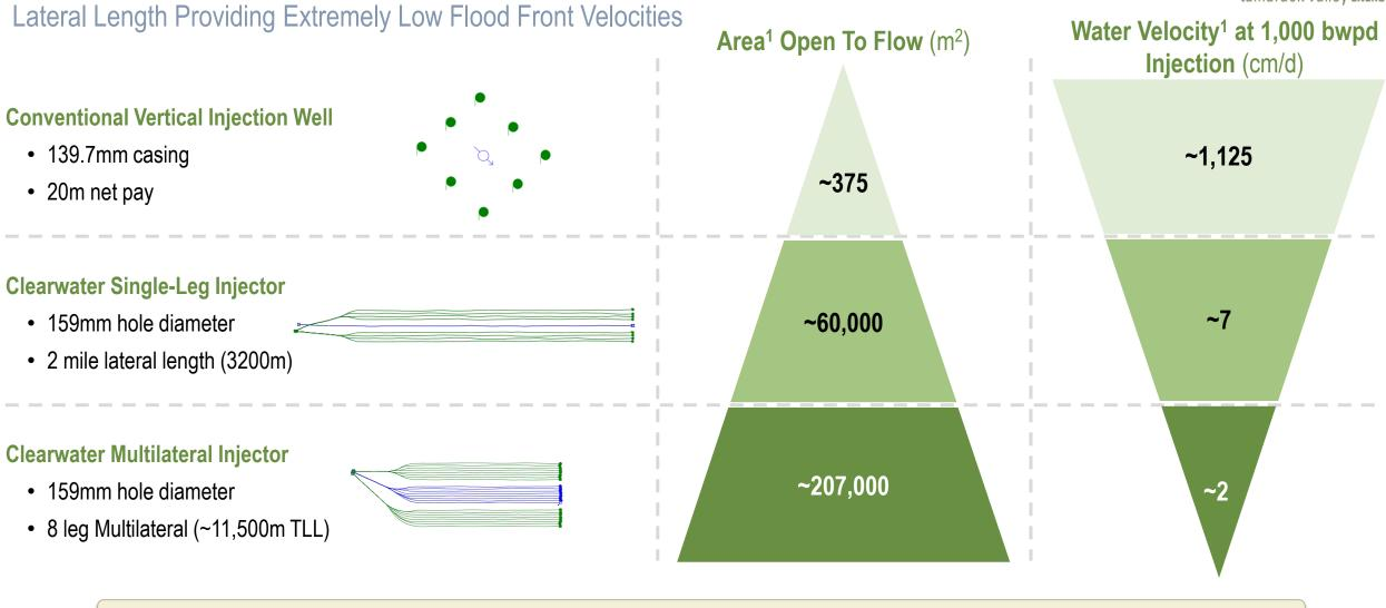
Horizontal and Multilateral Wells Provide Extremely Large Areas Open To Flow, Which Results In Extremely Low Fluid Velocities In The Reservoir
