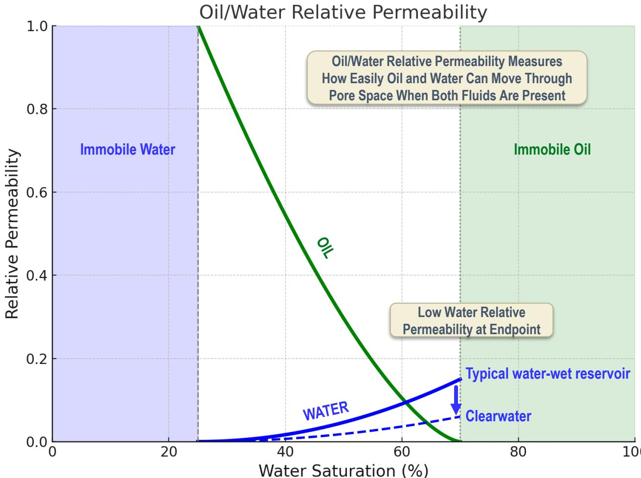
**Clearwater Reservoirs Have Low Relative Permeability To Water at The Endpoint (Residual Oil Saturation)**
