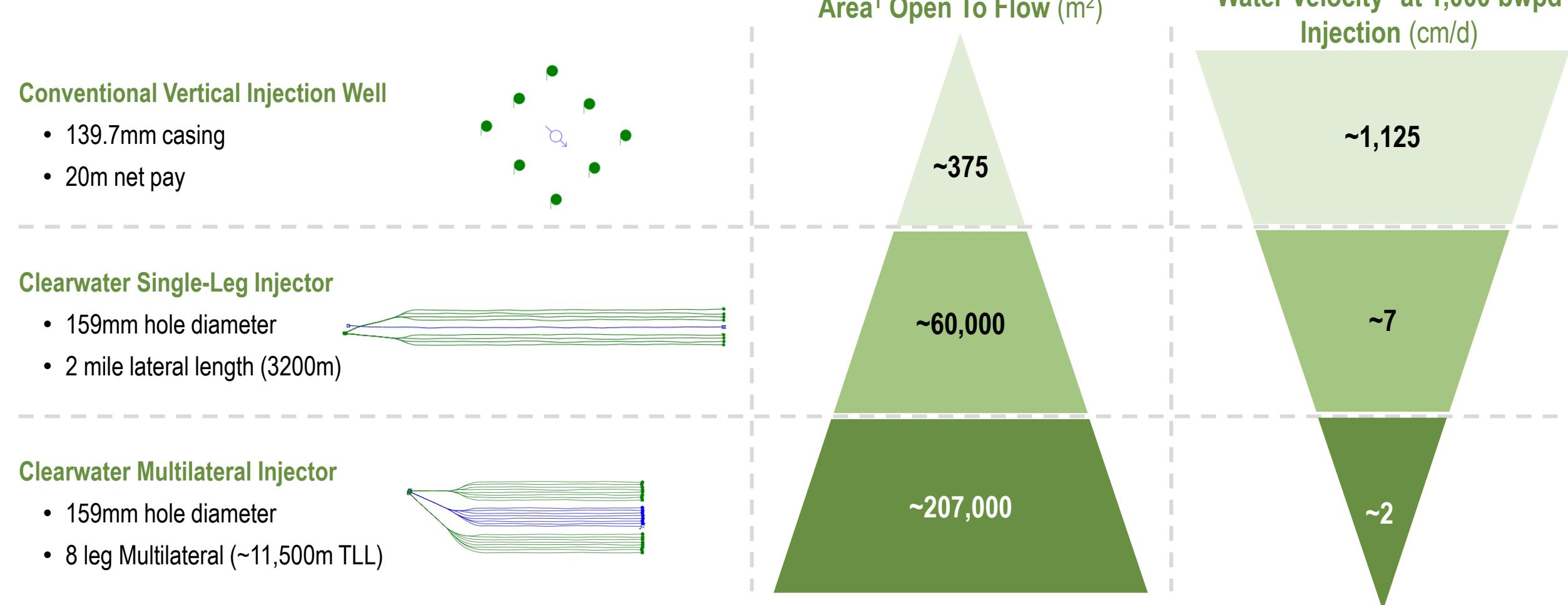
Horizontal and Multilateral Wells Provide Extremely Large Areas Open To Flow, Which Results In Extremely Low Fluid Velocities In The Reservoir
