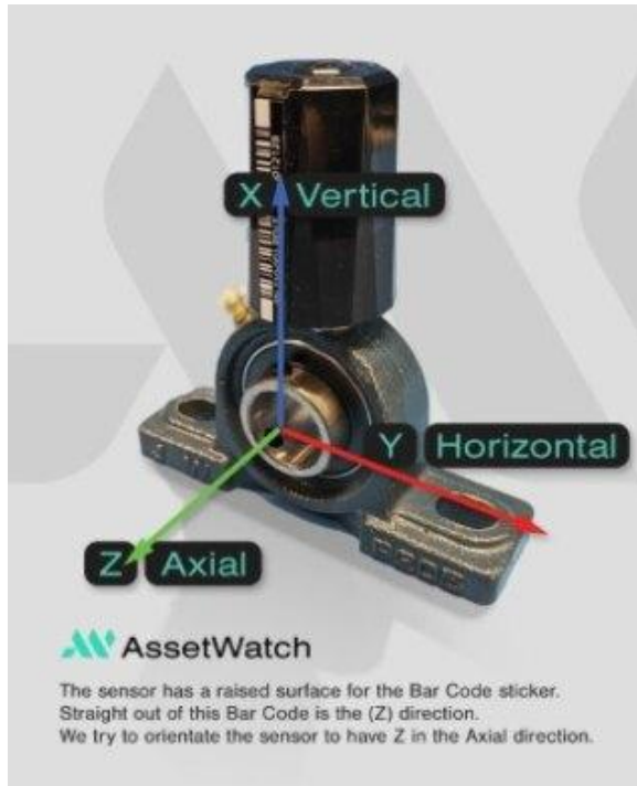
Figure 4: Example Orientation of Older Style PB-SM
