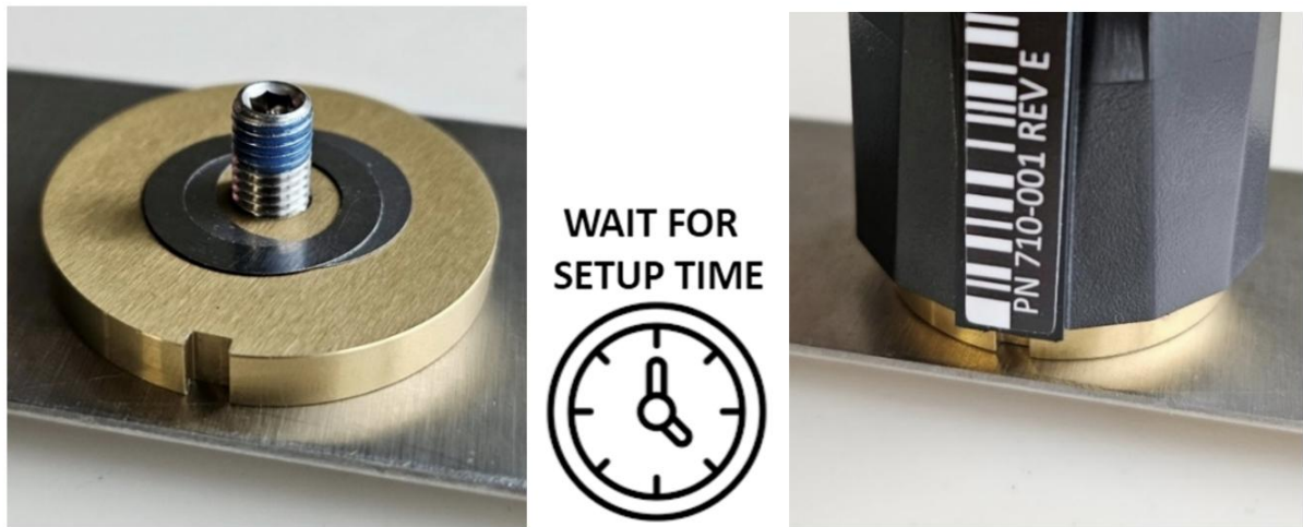
Figure 9: Instructions: Strike plate with threaded stud installation. Mount Sensor after epoxy is cured 30 Mins.
