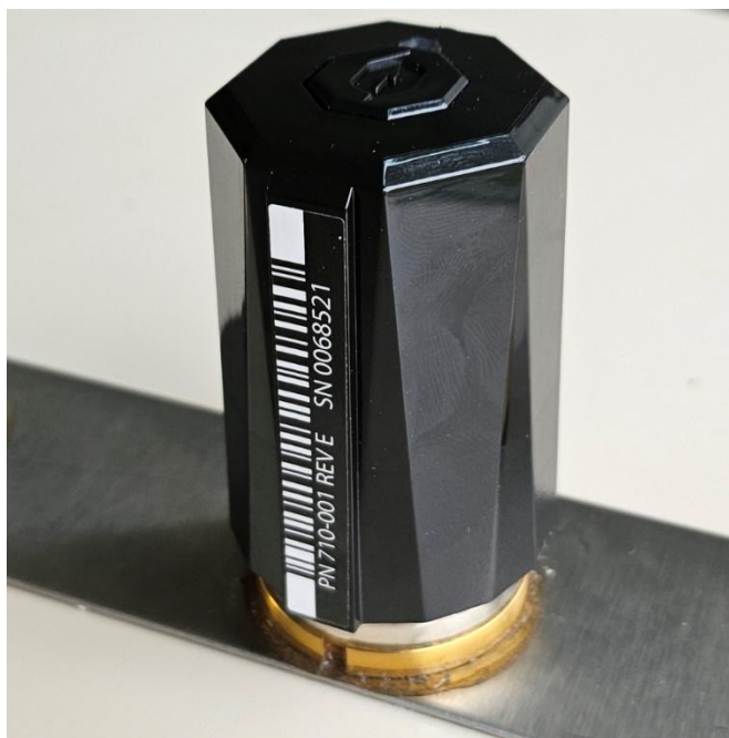
Figure 7: PB-SM alignment feature with strike plate notch
