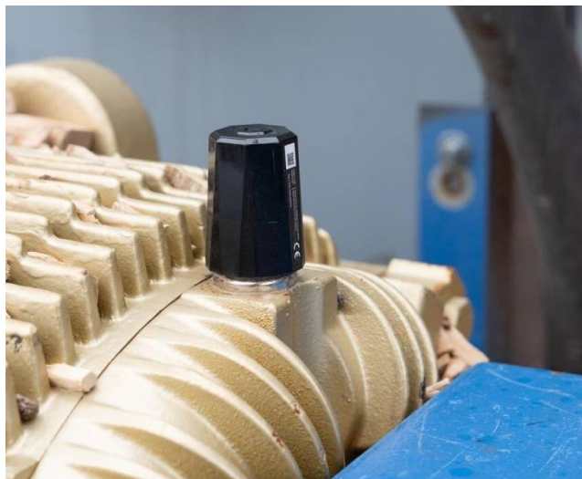
Figure 3: Typical PB-SM Installation with supplied magnet
