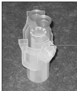
1.5 mL microcentrifuge tube lid in the wrong slot of the rotor adapter
