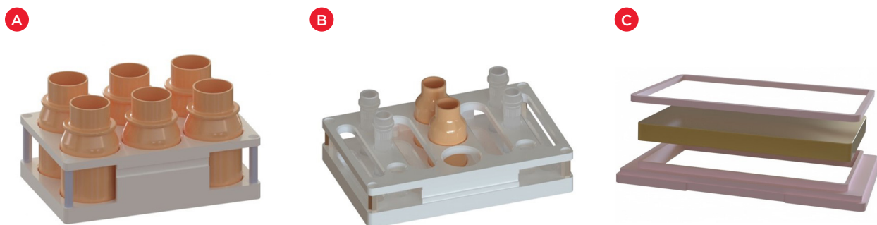
Figure 4. Customized labware: (A) rack with buffer vials, (B) rack with beads and digest vials, and (C) tissue holder with tissue for blotting.
