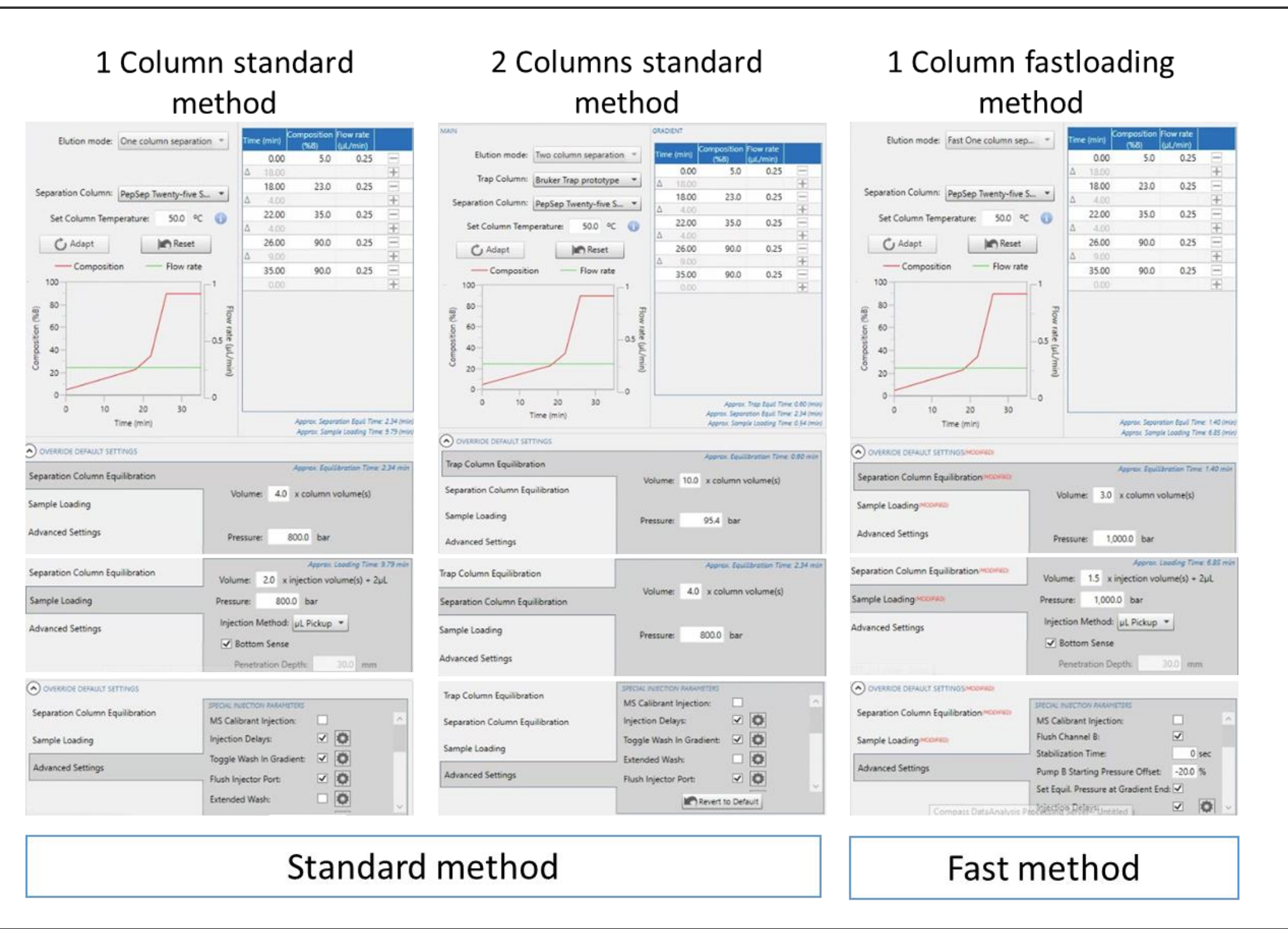
Fig. 2 Chromatographic methods setup. All three methods use the same 22 min active gradient method. They differ by there equilibration and loading protocols, namely the wash volume and equilibration / loading pressure. The total run time is 55 minutes for the 1C method, 47 minutes for the 2C method and the 1C fast loading method.
