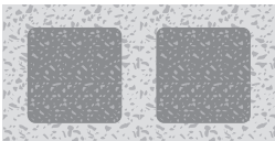
Block 12MPa, fine grout 20MPa
