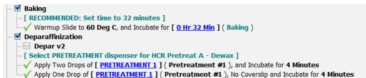
If you prefer baking slides offline, de-select **Baking**. **Pretreat A** must be placed into an open **PRETREATMENT dispenser**. Make sure that the **Pretreatment** selections are the same.
